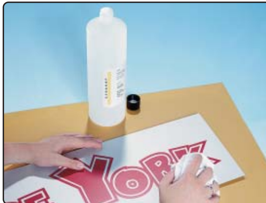
4. Finally clean with solvent or environmentally friendly GEDA Clean.
