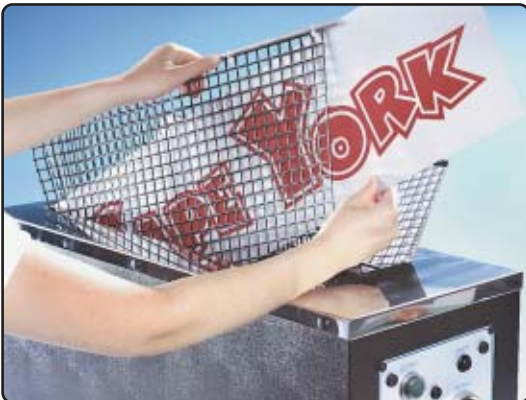
3. Close pores in GEDA Sealing Tank, minimum 40 minutes at 95°C / 203°F.
