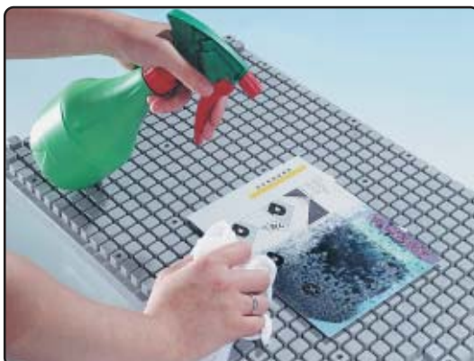
5. Strip with GEDA Stripper.
