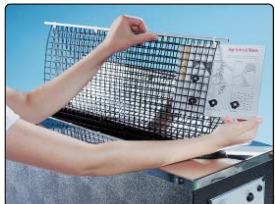
6. Close open pores in GEDA SealingTank, minimum 40 minutes at 95°C / 203°F. Finally clean with solvent or environmentally friendly GEDA Clean.
