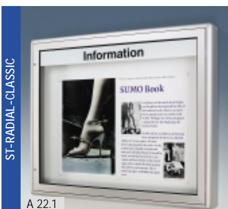
ST-RADIAL-CLASSIC Extruded aluminium profiles with cast aluminium corners. 80mm deep with 75mm border on glass frontage.
